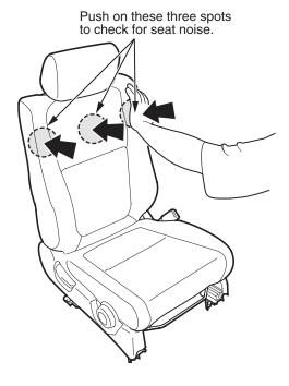
If you hear any noise, go to **REPAIR PROCEDURE** to repair the noisy seat.
