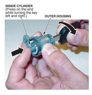
Using your thumb and forefinger to hold the tumblers, remove the key from the inner cylinder, being careful not to drop any tumblers and springs.
