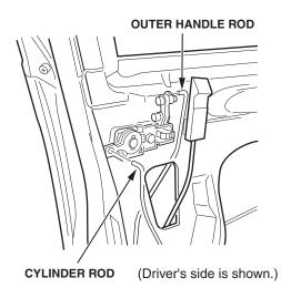
10. Pull down on the retainer clip with a hook-shaped tool. Remove the lock cylinder. Then go to step 14.
