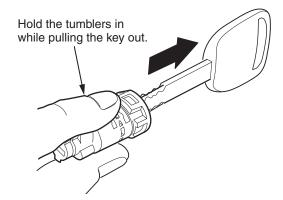
20. Using the key code from the *i*N that you have written down at step 2, build a new inner cylinder with new springs, new cylinder, and tumblers from the door lock cylinder kit. Make sure you put the appropriate numbered tumbler in the proper inner cylinder cavity. Apply a thin layer of Permalube to each tumbler to help lubricate and retain it.
