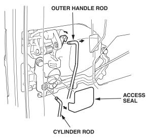
13. Push the top of the retainer clip with a flat-tip screwdriver, and hold it. Release the retainer clip with a hook-shaped tool, then remove the lock cylinder. Go to step 14.
