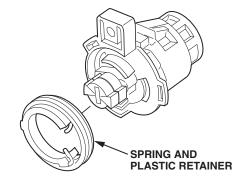
17. Using a small screwdriver, push down on the tip of the last tumbler to release it, then remove the cylinder from the housing, being careful not to drop any tumblers and springs. Use your thumb and forefinger to hold the tumblers in place. Then go to step 20.
