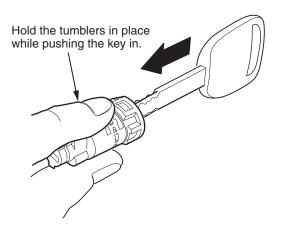
21. Leave the key in the cylinder. Reinstall the plastic retainer and spring if you removed them in step 16. Hold the plastic retainer and spring on the housing, and insert the inner cylinder. Rotate it left and right to engage the spring to the inner cylinder. Make sure the spring is properly seated to the inner cylinder.
