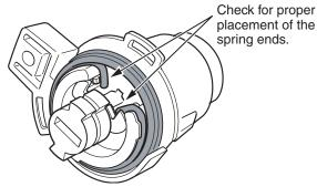
22. Install the arm with a new cylinder rod clip and a new E-clip.
