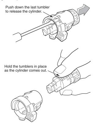
18. While turning the key left and right and pushing on the rear of the inner cylinder to release the spring, slowly remove the cylinder from the housing.
