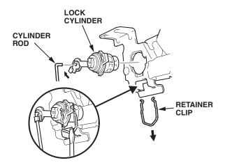
8. Release the clip, detach the hook, and remove the lock rod protector.
