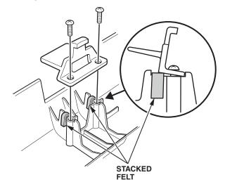
6. Install the seat trim cover, and check the trim cover latch for proper engagement.
