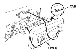
2. Remove the two screws that attach the trim cover latch to the rear seat trim cover.
