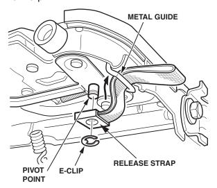
Install the seat support inner cover, making sure to feed the release strap through the slot in the cover.
