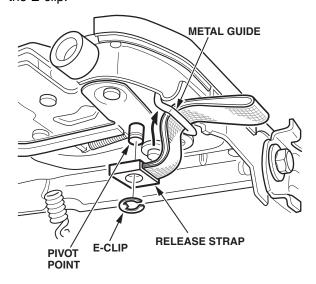
Install the seat support inner cover, making sure to feed the release strap through the slot in the cover.
