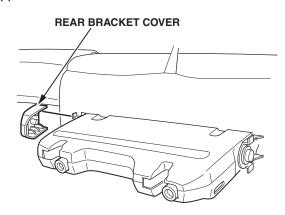
7. Wearing gloves and eye protection, carefully cut the plastic weld on the rear of the seat support covers with a utility knife. To cut the weld, insert the blade into the gap below the weld, and move the knife toward the pivot bolt.
