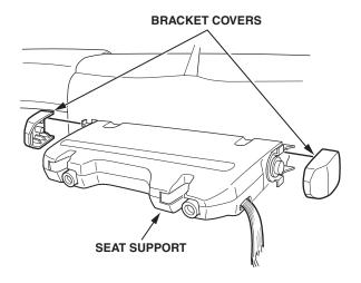
4. Wearing gloves and eye protection, carefully cut the plastic weld on both ends of the seat support covers with a utility knife. To cut the weld, insert the blade into the gap below the weld, and move the knife toward the pivot bolt.
